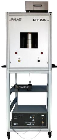
The MFP filter test rig is a modular filter testing system for flat filter media and small mini-filters. The MFP 2000 can be used to determine pressure loss curve on the medium without a dust coating, fraction separation efficiency, or burden and fraction separation efficiency during application of the burden within shortest times – reliably and therefore cost-effectively.
