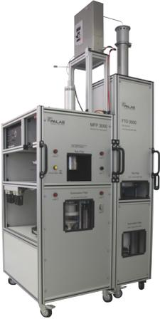
The MFP 3000 FTD filter test rig comprises the test rig MFP 3000 with a test surface of 100 cm<sup>2</sup> and the additional conduit FTD 3000 with a test surface of 400 cm<sup>2</sup>, which can be operated in turn.
