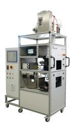
Version MFP 3000 G is especially tailored to the requirements of the ISO 16890 measurement procedure.
