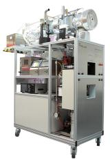
With the MFP 3000 HF, it is possible to set the relative humidity from 10 to 80 % or the temperature from -10 to 50 °C. The inflow velocity has been extended compared to standard models to a range of 4 cm/s – 2 m/s.
