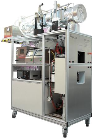
With the MFP 3000 HF, it is possible to set the relative humidity from 10 to 80 % or the temperature from -10 to 50 °C. The inflow velocity has been extended compared to standard models to a range of 4 cm/s – 2 m/s.
