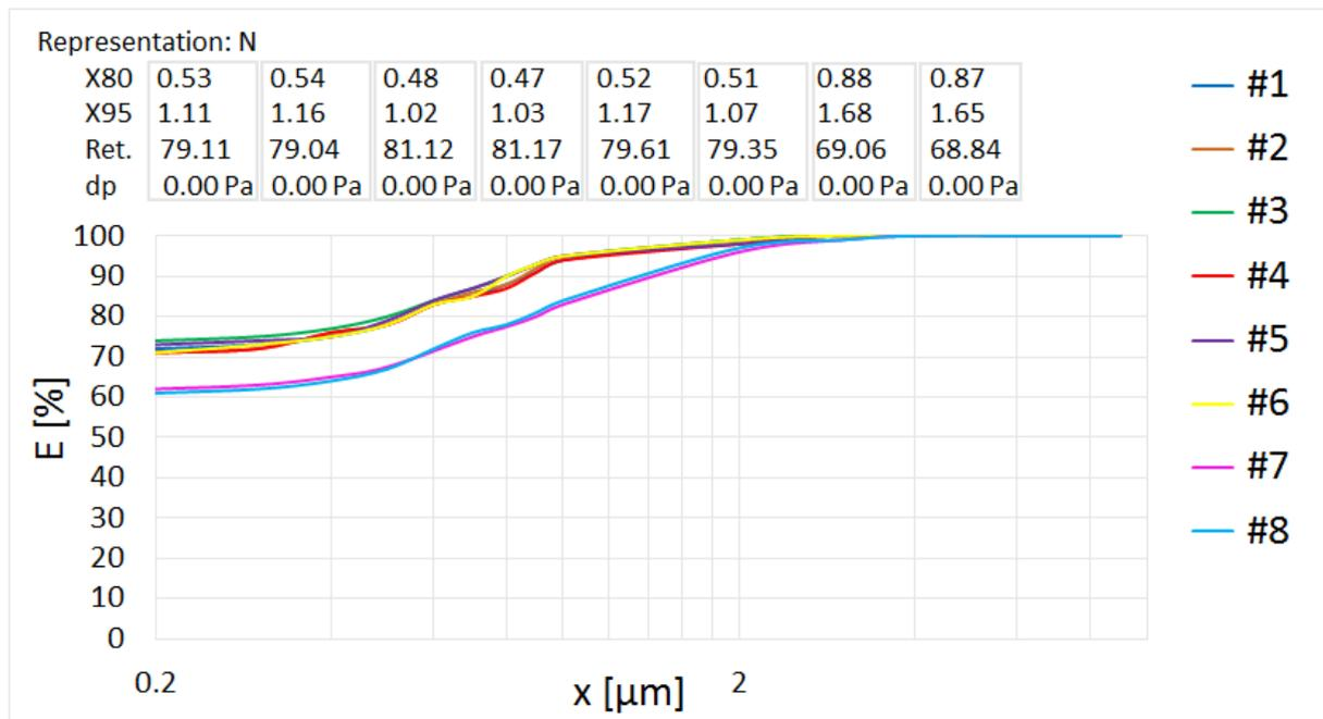
Fig. 2: Example: Comparison of fraction separation efficiencies
