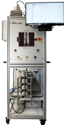
The MFP filter test rig is a modular filter testing system for flat filter media and small mini-filters.
