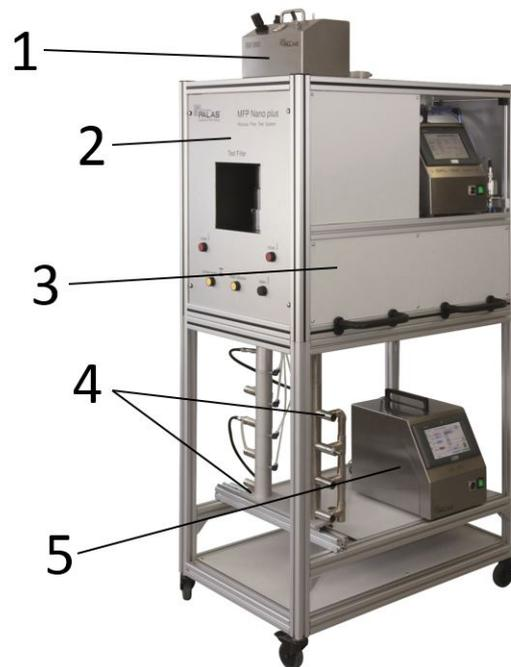
1. Variable aerosol generation with the UGF 2000 for KCl / NaCl or DEHS. We integrated silica gel drying length. The volume flow for aerosol generation is individually regulated via mass flow controllers.
