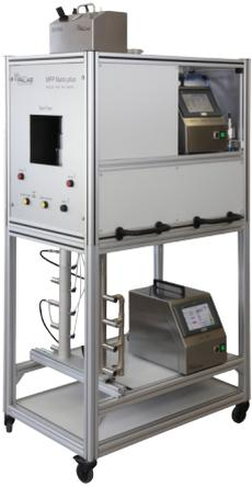
The MFP Nano *plus* has been specially designed to determine the separation efficiency of HEPA and ULPA filter media in accordance with DIN EN 1822-3 and ISO 29463-3. In the form of the U-SMPS, a modern and powerful nanoparticle measuring device with a measurement range from 5 nm to 1  $\mu\text{m}$  is used for particle size and quantity analysis.
