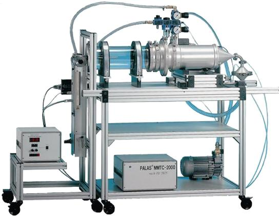
In this version, the filter holder MMTC 2000 E is made of V2A in order to cover a higher temperature range.
