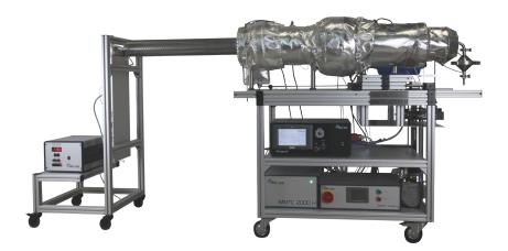
In this version, the filter holder MMTC 2000 E is made of V2A in order to cover a higher temperature range. The addition of heating and insulation allows filter testing at temperatures of up to  $250\,^{\circ}$ C.
