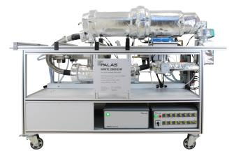
In this version, the filter holder MMTC 2000 EHF is made of V2A to cover a higher temperature range. Adding heating and insulation allows filter testing at temperatures up to 250 °C.
