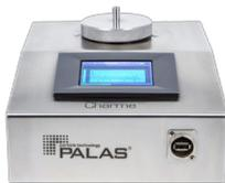
Charme® is a high-capacity Faraday cup aerosol electrometer that measures the electrical charges on aerosol particles. For years, aerosol electrometers have been used in research applications to measure the mean charge of an aerosol. If the charge state of the particles for monodisperse aerosols is known, then these devices can quickly and easily determine the number concentration of particles with an approx. size  $\geq 2$  nm.
