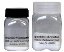
MP 20 are microparticles with a mean diameter of 20.56  $\mu m$ . The distribution of this dust is monodisperse; the geometric standard deviation of the distribution is only 4.56  $\mu m$ . Due to this small distribution, these dusts are used for scientific analysis and can also be used to calibrate measuring devices.
