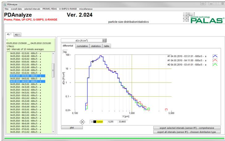
The PDANalyze software is designed to acquire measurement values and data analysis by all stand-alone particle measuring devices. It enables quick and easy analysis of particle sizes and concentrations using the Promo<sup>®</sup> System, Fidas<sup>®</sup> System, UF-CPC System, U-SMPS System, and U-RANGE System.
