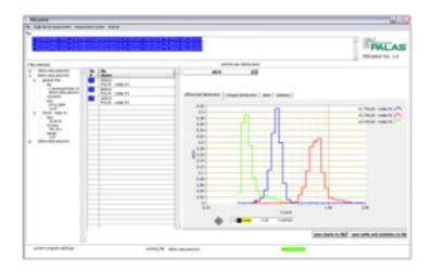
The PDControl software is designed for measurement value acquisition and data analysis by all the welas $^{\mathbb{R}}$  digital and Promo $^{\mathbb{R}}$  systems. It enables quick and easy particle size and concentration analysis.
