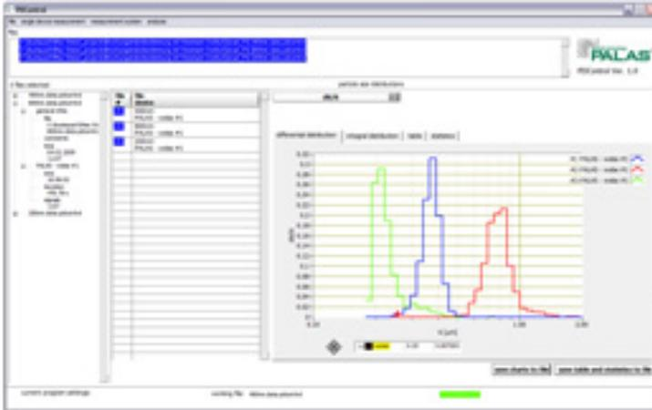
The PDCONTROL software is designed for measurement value acquisition and data analysis by all the welas<sup>®</sup> digital and Promo<sup>®</sup> systems. It enables quick and easy particle size and concentration analysis.
