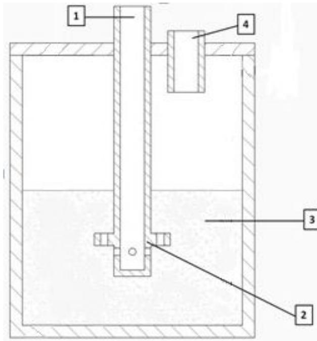
Fig. 2: Functional principle of the PLG series
