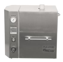
The PLG 2100 uses a nozzle system developed by Palas . Depending on the application, a special nozzle that is able to be heated to 120°C is used in order to enable quick and reproducible adjustment to the desired particle size distribution and concentration. Among other uses, the PLG 2100 is used on the HMT 1000 filter test rig to test oil nebulizers in order to disperse a corresponding motor oil, e.g. 10w-40.
