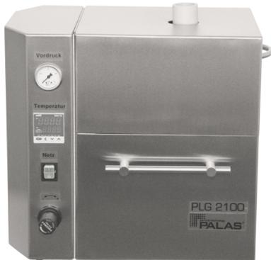
The PLG 2100 uses a nozzle system developed by Palas . Depending on the application, a special nozzle that is able to be heated to 120°C is used in order to enable quick and reproducible adjustment to the desired particle size distribution and concentration. Among other uses, the PLG 2100 is used on the HMT 1000 filter test rig to test oil nebulizers in order to disperse a corresponding motor oil, e.g. 10w-40.
