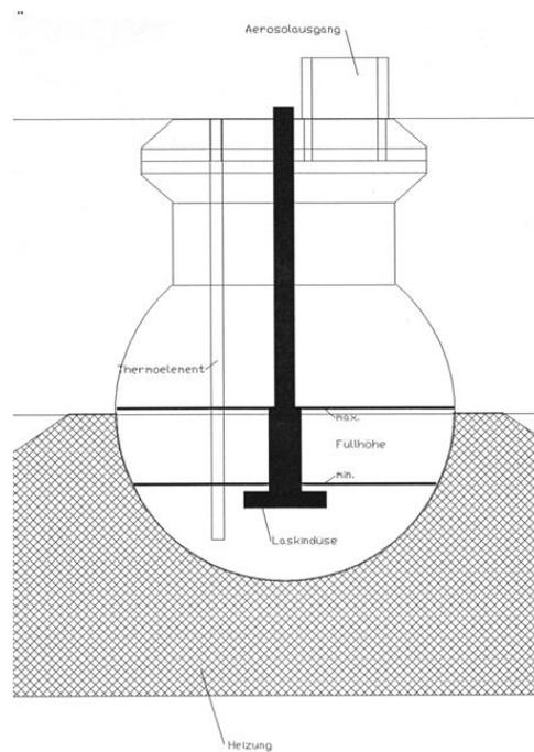
Fig. 1: Schematic diagram of the PLG 2100 aerosol generator
