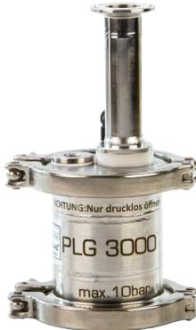
The PLG 3000 is used for fractional separation efficiency measurement and loading with oil aerosols as per ISO 12500-1. The oil quantity can be adjusted using the dispensing volume flow between approx. 0.2 – 12 g/h. The PLG 3000 aerosol generator is designed to be pressure-resistant up to 7 bar positive pressure (higher pressure values upon request).
