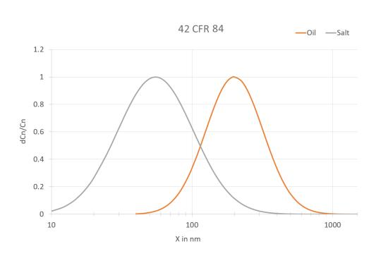
Based on the measurement of particle penetration via particle size, the PMFT 1000 F can also be used to consider the tolerances in the particle size distribution according to EN 13274-7 as a min. / max. penetration value.
