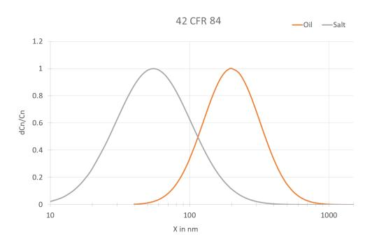
Based on the measurement of particle penetration via particle size, the PMFT  $1000\,\mathrm{F}$  can also be used to consider the tolerances in the particle size distribution according to EN 13274-7 as a min. / max. penetration value.
