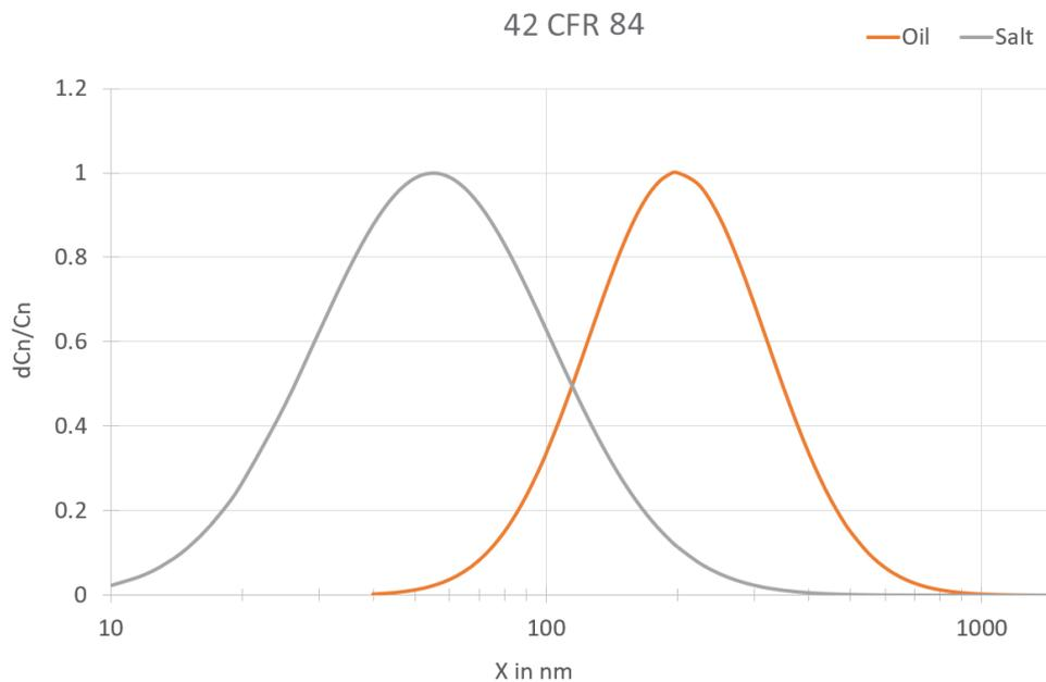
Based on the measurement of particle penetration via particle size, the PMFT 1000 F can also be used to consider the tolerances in the particle size distribution according to EN 13274-7 as a min. / max. penetration value.
