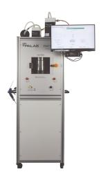
The PMFT 1000 M tests face masks better than the standards EN 149/EN 13274-7 with additional accurate analysis of filter mask efficiency for SARS-CoV-2 (size approximately 120 nm to 160 nm). Both total photometric penetration and fractional efficiency are tested, e.g., the efficiency in the whole size range, respectively, the particle size-dependent penetration.
