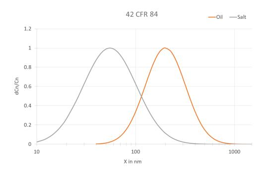
Based on the measurement of the particle penetration via the particle size, the PMFT 1000 M can also be used to consider the tolerances in the particle size distribution according to EN 13274-7 as min./max. penetration value. In addition, comparative values to other manufacturers are possible (option).
