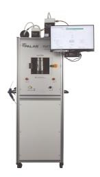
The PMFT 1000 tests respirators better than the standards EN 149/EN 13274-7 with additional accurate analysis of filter mask efficiency for SARS-CoV-2 (size approximately 120 nm to 160 nm). Both total photometric penetration and fractional efficiency are tested e.g., the efficiency in the whole size range respectively the particle size-dependent penetration.
