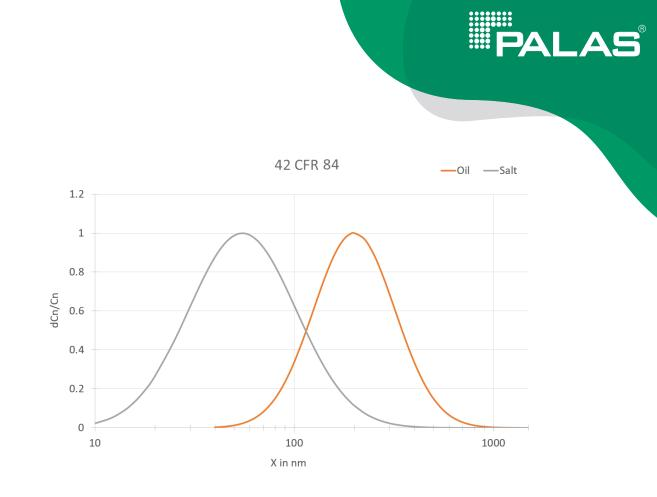
Based on the measurement of the particle penetration via the particle size, the PMFT 4000 can also be used to consider the tolerances in the particle size distribution according to EN 13274-7 as min. / max. penetration value.
