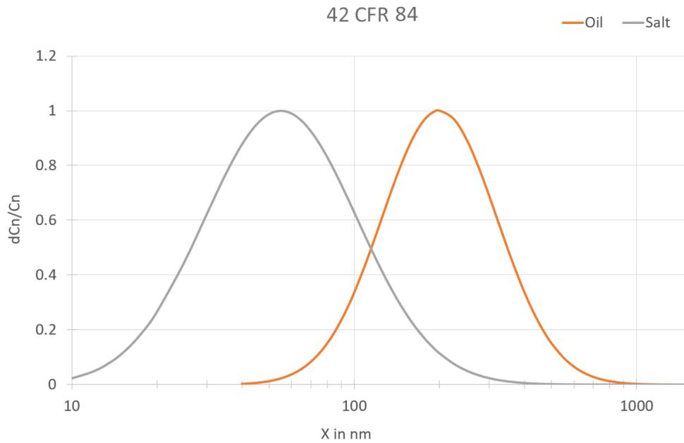
Based on the measurement of the particle penetration via the particle size, the PMFT 4000 can also be used to consider the tolerances in the particle size distribution according to EN 13274-7 as min. / max. penetration value.
