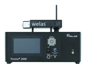
The welas<sup>®</sup> aerosol sensors welas<sup>®</sup> 2070 P, 2100 P, 2300 P and welas<sup>®</sup> 2500 P are equipped with a pressure-tight cuvette to ensure isobaric and isothermal sampling into the sensor's measurement volume. The Promo<sup>®</sup> system is usually calibrated for the operating volume flow. As the operating volume flow changes with pressure, it is advantageous for the user if automatic volume flow regulation for the sampling volume flow is provided for in the device.
