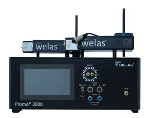
The welas aerosol sensors welas 2070 P, HP, 2100 P, HP, 2200 P, HP, 2300 P, HP and welas 2500 P, HP are equipped with a heatable and, as required, pressure-tight cuvette to ensure isobaric and isothermal sampling into the sensor's measurement volume. The Promo 3000 H model variant also offers heating regulation for temperatures up to 250 °C for the aerosol sensors with heatable cuvette. The Promo system is usually calibrated for the operating volume flow.
