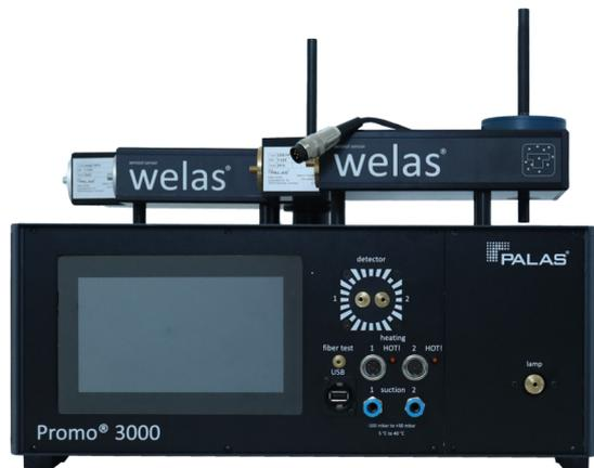
The welas<sup>®</sup> aerosol sensors welas<sup>®</sup> 2070 HP, 2100 HP, 2300 HP, and welas<sup>®</sup> 2500 HP are equipped with a cuvette heatable up to 120 °C and pressure-tight up to 10 barg to ensure isobaric and isothermal sampling into the sensor's measurement volume.
