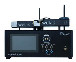
The welas  $^{\$}$  aerosol sensors welas  $^{\$}$  2070 HP, 2100 HP, 2200 HP, 2300 HP, and welas  $^{\$}$  2500 HP are equipped with a cuvette heatable up to 120  $^{\circ}$ C and pressure-tight up to 10 barg to ensure isobaric and isothermal sampling into the sensor's measurement volume.
