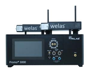
The welas  $^{\mathbb{R}}$  aerosol sensors welas  $^{\mathbb{R}}$  2070 P, 2100 P, 2200 P, 2300 P, and welas  $^{\mathbb{R}}$  2500 P are equipped with a pressure-tight cuvette to ensure isobaric and isothermal sampling into the sensor's measurement volume.
