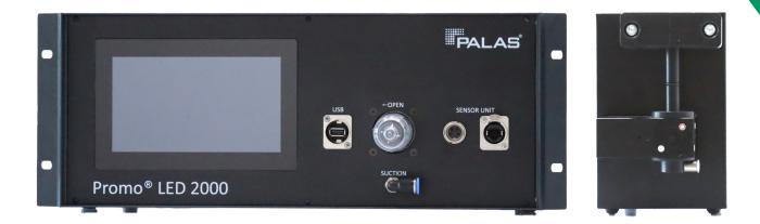
The new light-scattering aerosol spectrometer Promo<sup>®</sup> LED 2000can be equipped with different sensors for particle size analysis and concentration determination from 0.145 to 100  $\mu$ m can be fitted with different sensors. The heart of the optical sensors is the new LED technology with an extra-long lifetime at the highest stability in particle sizing and counting applications.
