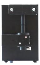
The new light-scattering aerosol spectrometer Promo® LED 2000can be equipped with different sensors for particle size analysis and concentration determination from 0.145 to  $100~\mu m$  can be fitted with different sensors. The heart of the optical sensors is the new LED technology with an extra-long lifetime at the highest stability in particle sizing and counting applications.
