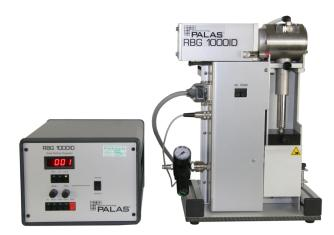
The dispersion unit and the electrical control unit can be set up up to 2 m apart from each other. The return speed for container changeover is optimized on the RBG 1000 I and is faster than on the other RBG variants. It is only approx. 1 minute.
