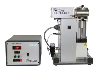
This device disperses particles at positive pressure values of up to 3 bar. The dispersion unit and the electrical control unit can be set up up to 2 m apart from each other. The return speed for container changeover is optimized on the RBG 1000 I and is faster than on the other RBG variants. It is only approx. 1 minute.
