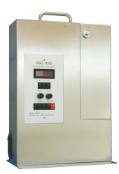
This device disperses particles at positive pressure values of up to 3 bar and can also use nitrogen and air as the dispersing gas.
