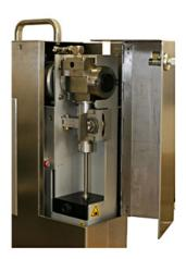
This version is equipped with special dispersion covers (type A, type B) and special solid material reservoirs with diameters of 7, 10, and 14 mm.
