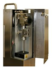
This version is equipped with special dispersion covers (type A, type B) and special solid material reservoirs with diameters of 7, 10, and 14 mm.
