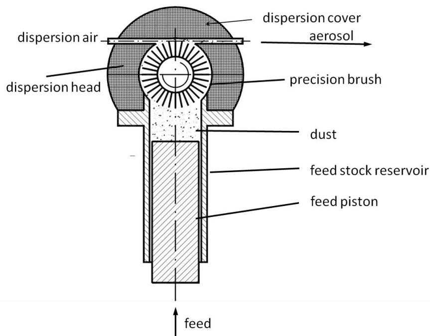
Fig. 1: RBG system schematic diagram
