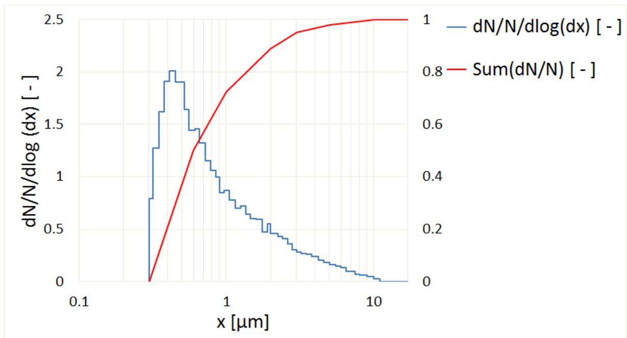
Fig. 2: Particle size distribution with welas<sup>®</sup> digital 2000
