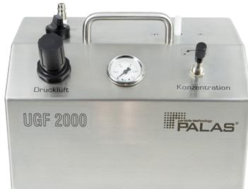
The UGF 2000 aerosol generator can atomize liquids with a binary nozzle.
