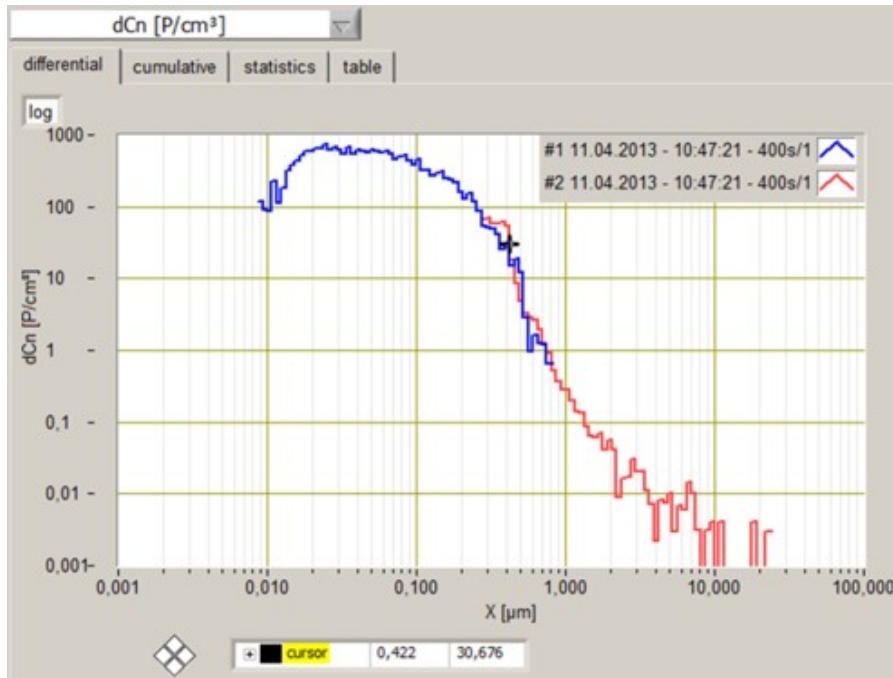
Figure 4: PDAnalyze evaluation software Measurement of indoor air concentration and display of number concentration Blue: Data from the U-SMPS, red: Data from the Fidas®
