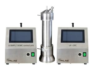
A soft X-ray source as a neutralizer is already integrated. The advantage instead of a radioactive neutralization (for example, with Kr-85) is that there is no need to follow requirements during transportation.
