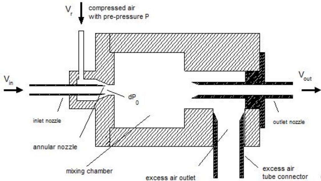
Particle-free air with the volume flow  $\dot{V}_R$  circulates through an annular passage around the suction nozzle. Thus, according to Bernoulli, a volume flow  $\dot{V}_{An}$  is generated at the suction nozzle.
