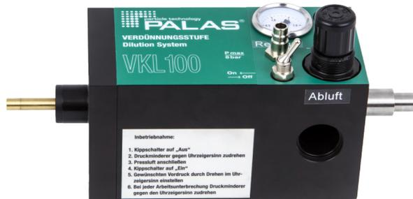
The VKL 100 series of dilution systems can reduce the concentration of aerosols by the dilution factor 1:100, also of very highly concentrated aerosols, in a defined and reliable way.
