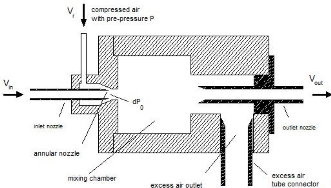
Particle-free air with the volume flow  $\dot{V}_R$  circulates through an annular passage around the suction nozzle. Thus, according to Bernoulli, a volume flow  $\dot{V}_{An}$  is generated at the suction nozzle. The dilution factor  $V_F$  is calculated according to the following formula.
