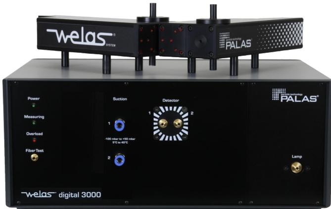
The aerosol sensors welas<sup>®</sup> 2070 P, 2100 P, 2200 P, 2300 P, and welas<sup>®</sup> 2500 P are equipped with a pressure-tight cuvette to ensure isobaric and isothermal sampling into the sensor's measurement volume.
