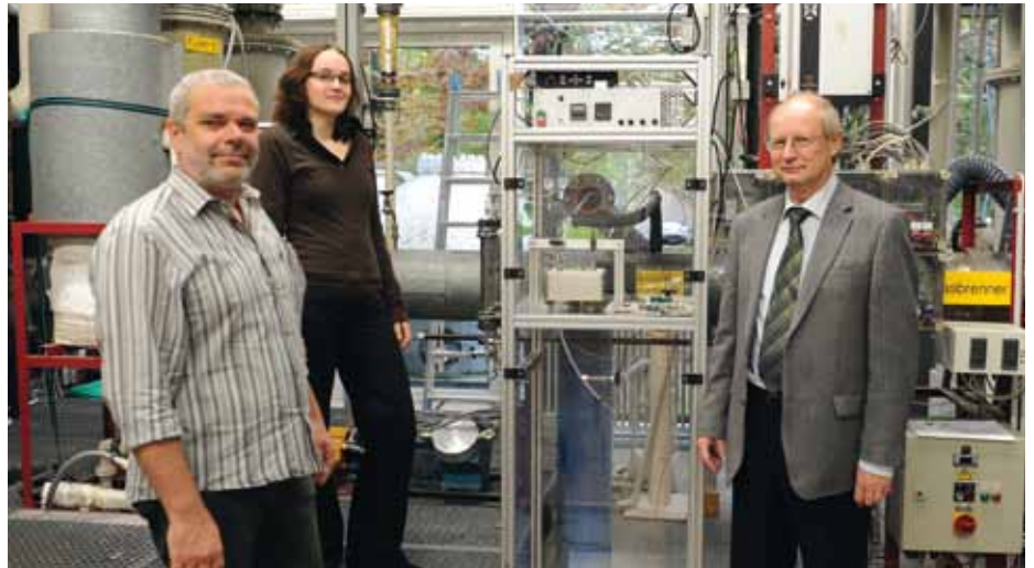
Dr. Sinanis, Dipl.-Ing. Brachert and Prof. Schaber in front of the flue gas system of the KIT. The measurement system consists of a Palas® dilution cascade DC 10000 iP, a welas® CNC module and an aerosol spectrometer welas® 2000 with control unit and aerosol sensor welas® 2070.
