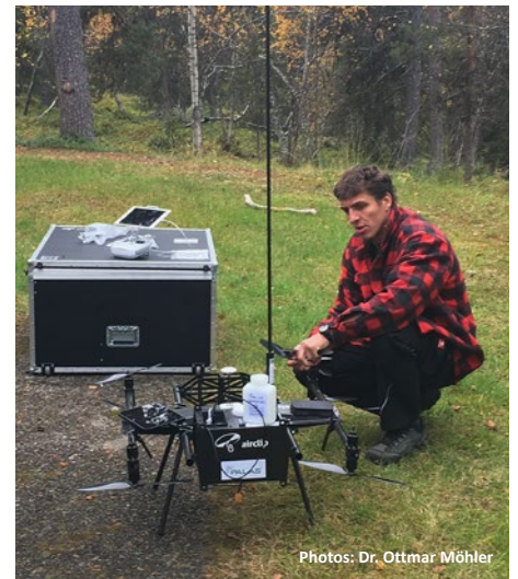
Drone pilot Gerd Schaufelberger with the Fidas® Fly 100 on the HORUS multicopter from Airclip
