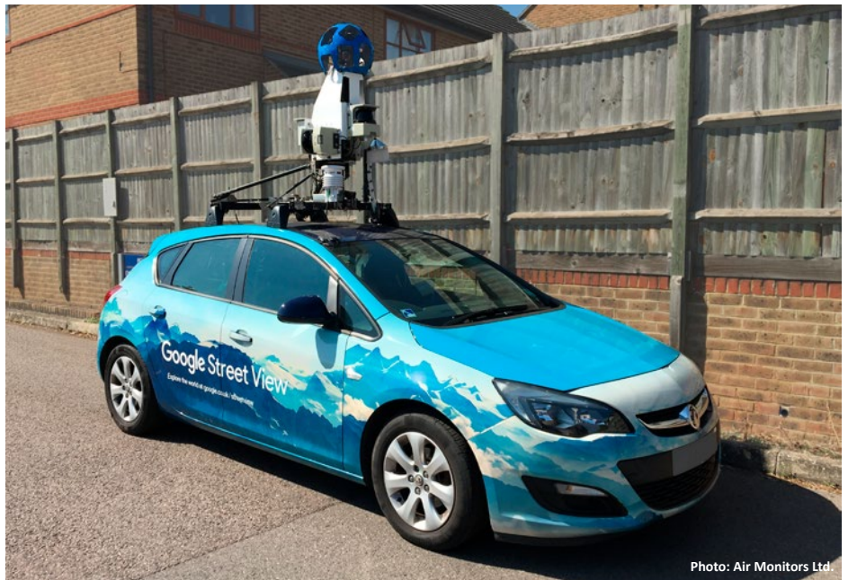
The Google Street View vehicle equipped with the Fidas® fine dust measurement device
