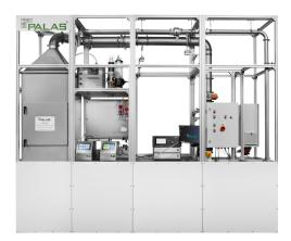
The FET 600 enables defined testing of filter elements up to 610 • 610 mm, such as ventilation filters, HEPA/ULPA filters, vacuum cleaner filters, and car cabin filters. Designed for optimum flow guidance, the channel can also use adapters for smaller filter elements. Coarse filters up to ULPA filters are tested for separation via particle size and differential pressure.
