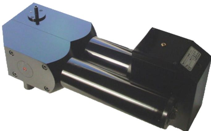
The model 1200 aerosol sensors are equipped with a small measurement volume and are used for coincidence-free measurement with a maximum number of concentrations of up to 50,000 particles/cm<sup>3</sup>. Measuring range: 0.12 – 3.5 μm / 0.2 – 10 μm / 0.3 – 17 μm / 0.6 – 40 μm.
