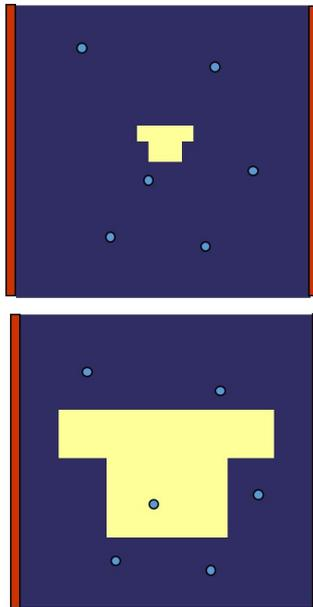
For concentrations up to 500,000 particles/cm<sup>3</sup>, the welas<sup>®</sup> 1100 sensor with a very small measuring volume is used. This ensures the smallest measuring volume such that only one particle ever enters the measuring volume. In low concentrations, the model welas<sup>®</sup> 1200 with a larger measuring volume offers the advantage of a higher counting rate at the same number concentration.
