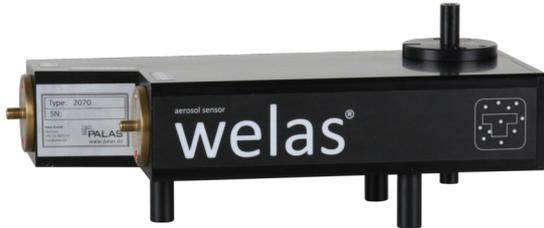
The model 2070 aerosol sensors are equipped with a very small measurement volume and are used for coincidence-free measurement with a maximum number of concentrations up to 1,000,000 particles/cm<sup>3</sup> and in the highest mass concentrations, e.g., Arizona dust A2, SAE Fine, up to 1,000 mg/m<sup>3</sup>. Measuring range: 0.2 – 10 μm / 0.3 – 17 μm / 0.6 – 40 μm.
