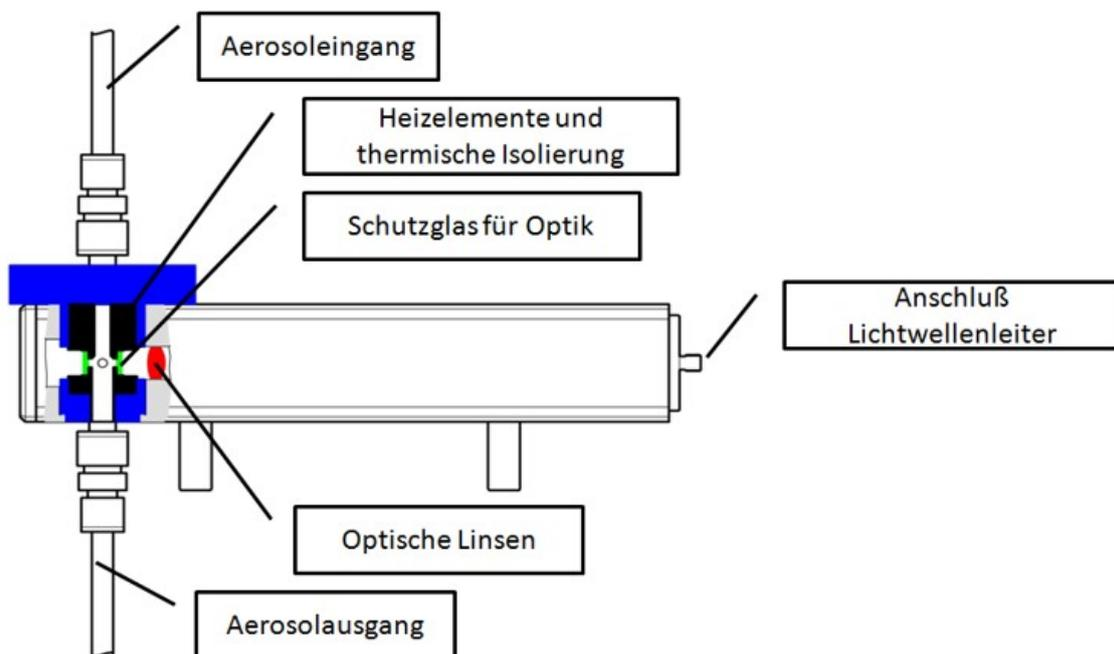
The table below shows the theoretical minimum separation of the particles at a given number concentration. At a number concentration of  $10^3$  per  $\text{cm}^3$ , the optical measuring volume must not be larger than  $1 \text{ mm}^3$ .
