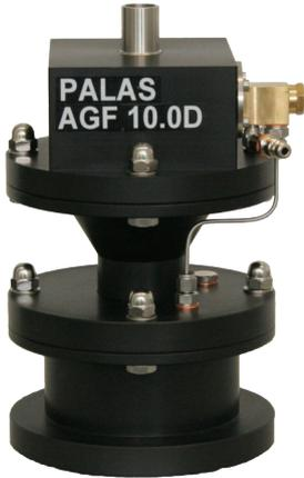
In contrast to the AGF 10.0, the AGF 10.0 D is pressure-resistant up to 10 bar overpressure and can therefore be used in applications with an absolute pressure of up to 11 bar, e.g. for testing compressed air filters and optical flow measurement methods in overpressure up to 10 bar.
