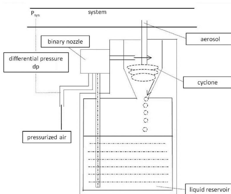
Fig. 1: Schematic diagram of the aerosol generator
