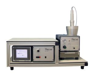
This dispersion system can continuously generate low mass flows, e.g.,  $8\,g/h$ , with optimal dosing constancy and control with automatic mass flow monitoring. Mass flow setting of approx.  $8\,g/h - 550\,g/h$  based on SAE fine, A2 dust.
