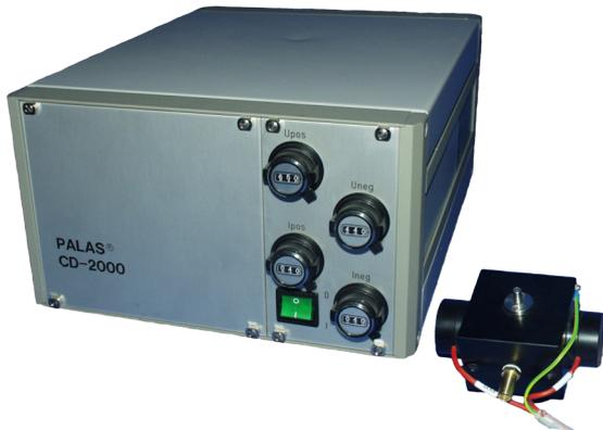
The CD 2000 type B bipolar discharge unit uses a mixed airflow of 3 – 36 m<sup>3</sup>/h with a tube diameter on the aerosol inlet of Ø<sub>i</sub>= 13 mm.
