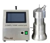
A soft X-ray source as a neutralizer is already integrated. The advantage instead of a radioactive neutralization (for example, with Kr-85) is that there is no need to follow requirements during transportation.
