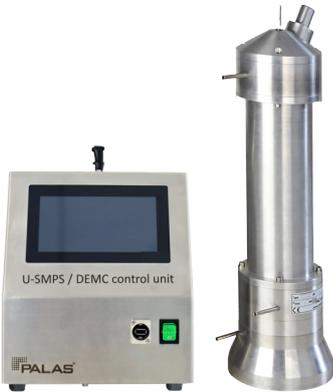
The DEMC size classifier (as defined in ISO 15900) selects aerosol particles based on their electrical mobility and directs them to the outlet. It is also often referred to as a DMA.
