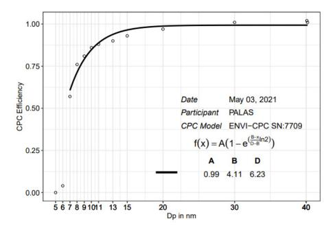
Fig. 1: Counting efficiency curve of the ENVI-CPC system measured at the Leibniz Institute for Tropospheric Research
