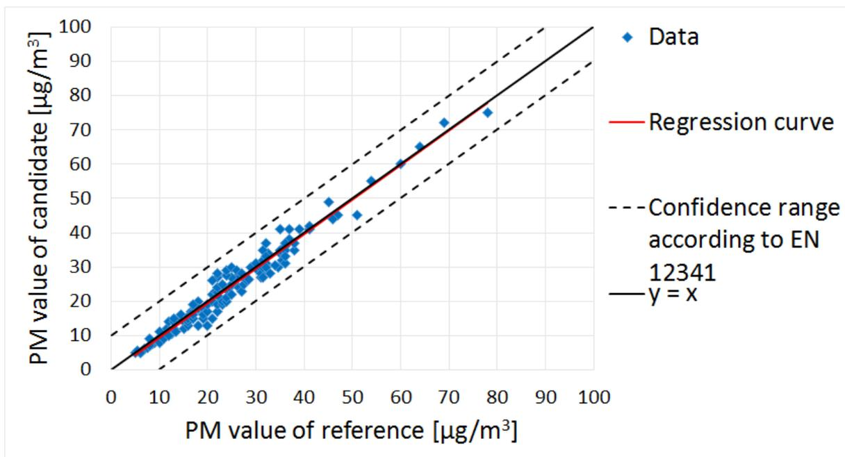
Fig. 3: PM<sub>10</sub> reference equivalence function of the Fidas<sup>®</sup> 200 S in comparison with a reference small-filter device during suitability testing from the "Report on supplementary testing of the Fidas<sup>®</sup> 200 S respectively Fidas<sup>®</sup> 200 measuring system manufactured by Palas GmbH for the components suspended particulate matter PM<sub>10</sub> and PM<sub>2,5</sub>, TÜV report no.: 936/21227195/B".
